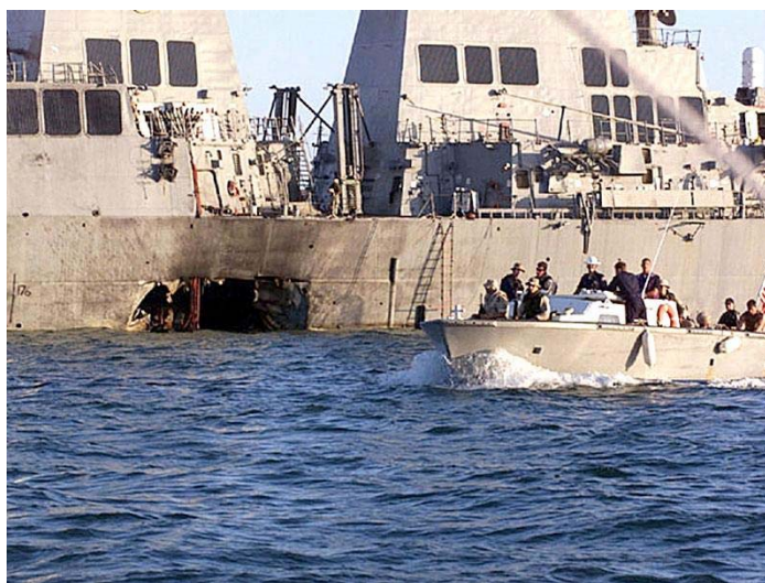
Figure 5-2. Suicide Bomb Damage to USS Cole . (Source: U.S. Navy)
